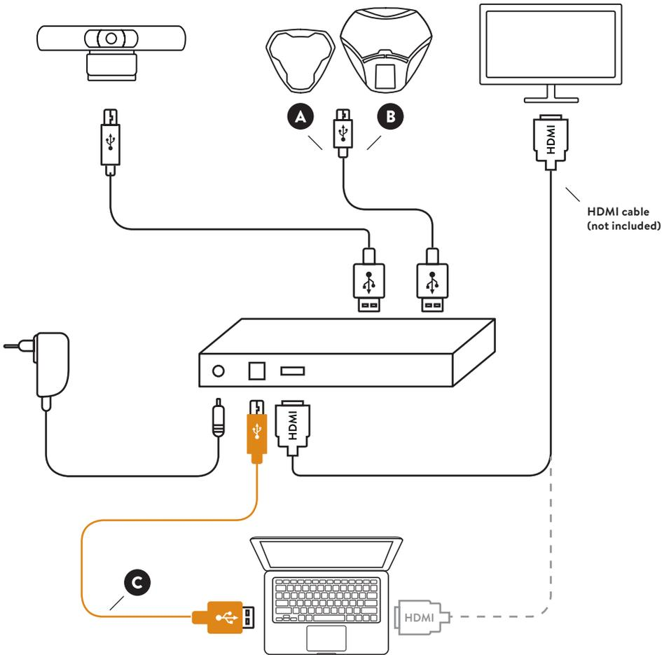
ⓘ Before connecting the USB cable **C** to the laptop, make sure that the DisplayLink driver is installed on the laptop.
